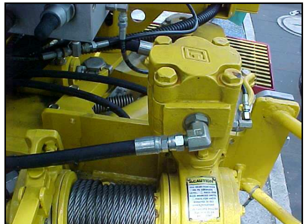
Figure 2 – 100K Pull-back Winch Lines
